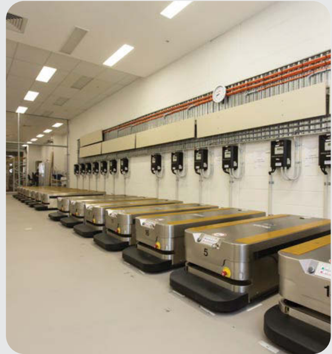
Automated guided vehicles docked at charging station
